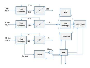
Figure 1. Pilot plant process design. UF = ultrafiltration, RO = reverse osmosis, HEX = heat exchanger.
