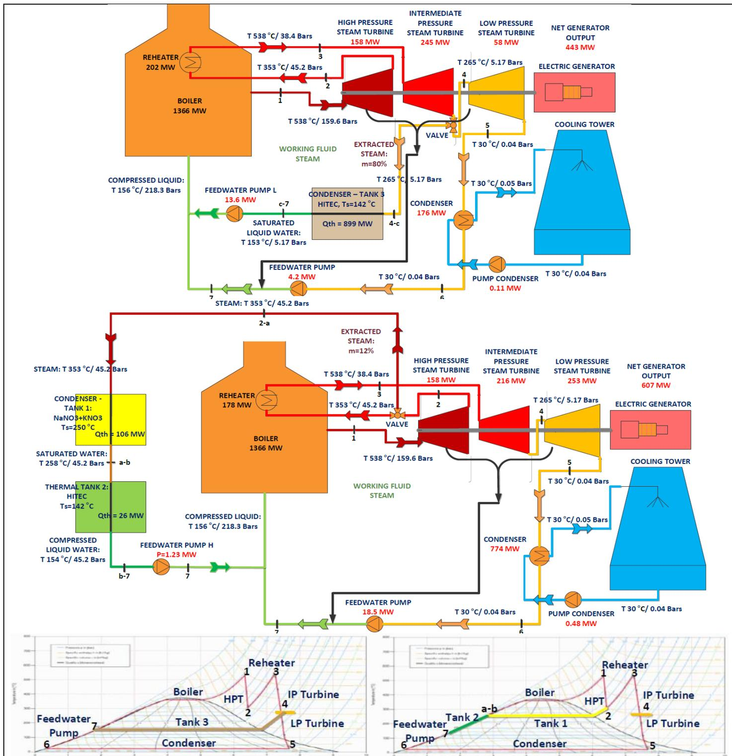
Fig. 2. Integration of: (top) two PCM-based TES tanks with steam extracted before the reheater, (middle) PCM-based TES tank with steam extracted before the LPT in the EDF nuclear power station, and (bottom) corresponding  $T$ - $S$  diagrams for the two cases.
