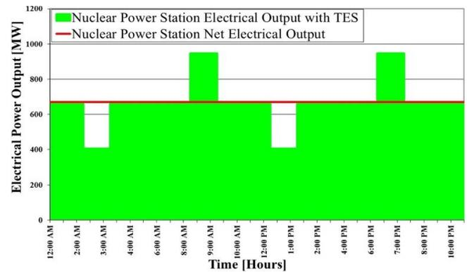
Fig. 1. Baseline net electrical energy production from the nuclear power station (670 MW) and electrical energy production after integration of the TES system.
