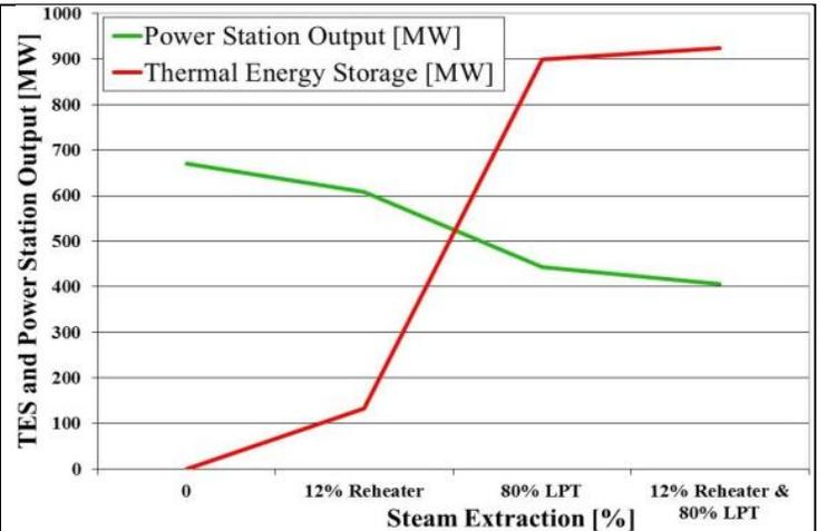
Fig. 3. Fractional plant derating, of main/base nuclear power station and stored thermal energy during TES charge, for the three EMS schemes proposed herein.
