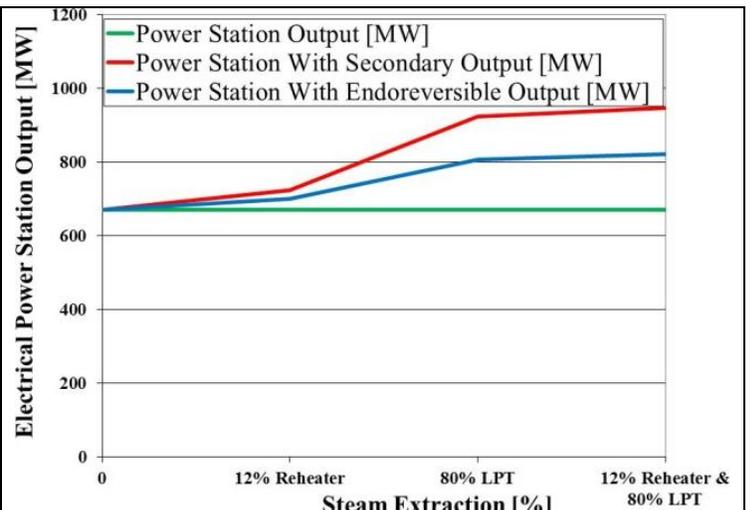
Fig. 5. Main/base nuclear power-plant output during TES charge, secondary (reversible) power output during TES discharge.
