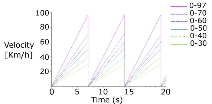
Fig. 2. Constant acceleration driving profiles
