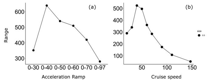
Fig. 4. Driving range for acceleration ramps and cruise speeds
