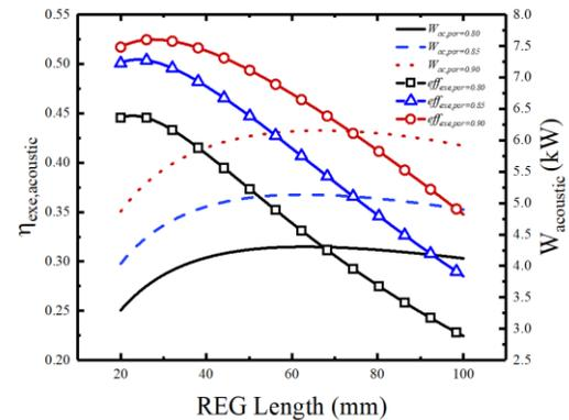
Fig 2 The effect of REG length and porosity on the system performance
