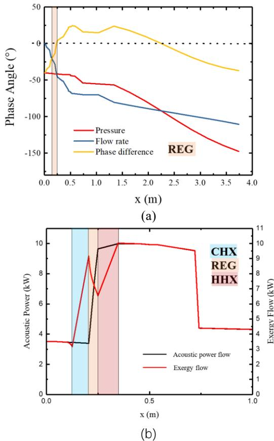
Fig 5 (a)Phase of pressure oscillation and flow rate;
