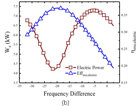
Fig 4 (a)Working frequency and LA's resonant frequency with different Spring stiffness;(b)System performance with the difference between LA's resonant frequency and system working frequency
