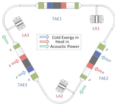
Fig 1 Schematic of the looped three-stage traveling-wave thermoacoustic generator system
