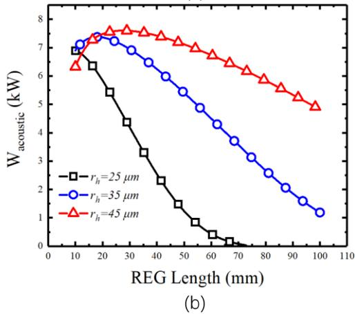
Fig 3 (a)Exergy efficiency of acoustic and (b) acoustic power output of one of three stages vary with hydraulic radius in different REG length
