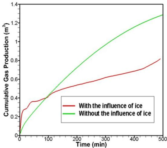
Fig 3 Comparison of the cumulative gas production over time with and without ice effects
