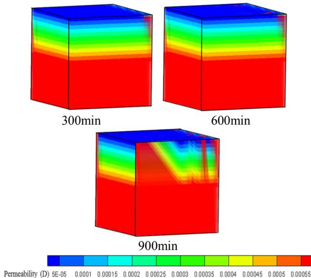
Fig 2 The absolute permeability change over time
