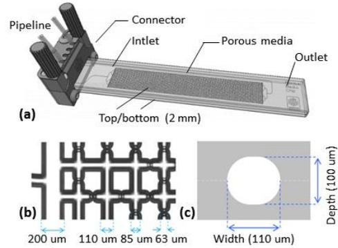
Fig 2 Microfluidic chip sample. (a) 3D overall structure picture; (b) size of local pores and throats; (c) a typical channel profile on the chip.
