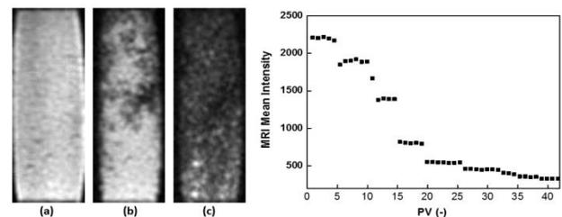
Fig 3 CO<sub>2</sub> drainage process at core scale (left; Ca=4.35×10<sup>-8</sup>); MRI mean intensity varies with injection CO<sub>2</sub> volume.
