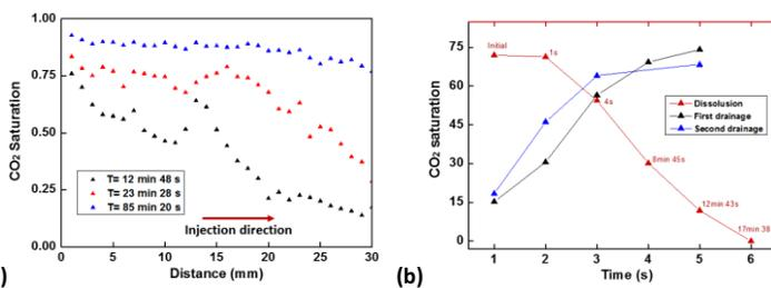
Fig 5 CO<sub>2</sub> Saturation distribution. (a) CO<sub>2</sub> saturation profiles at core scale; (b) variation in the CO<sub>2</sub> saturation with time at pore scale
