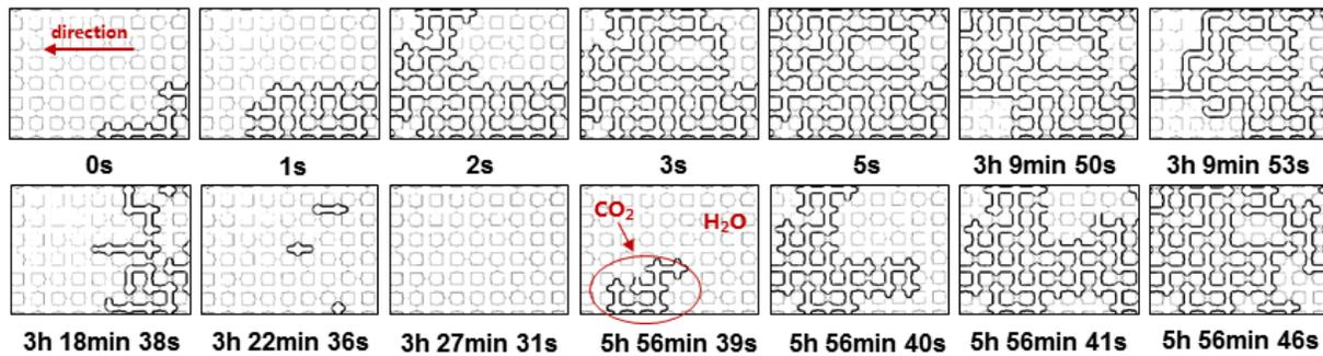
Fig 4 CO<sub>2</sub> drainage process at pore scale ( $Ca=5.3 \times 10^{-7}$ ). The area bounded by black line represents CO<sub>2</sub>. The porous region was saturated with water completely in the initial.
