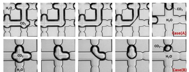
Fig 6 CO<sub>2</sub> dissolution morphology after first drainage under 6MPa. channel separate into two single CO<sub>2</sub> bubbles after
