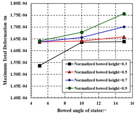
Fig. 8 Effect of bowed parameters on deformation of rotor
