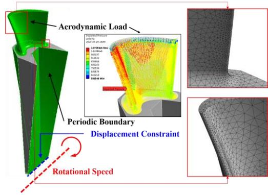
Fig. 4 FEA model of the turbine in present study
