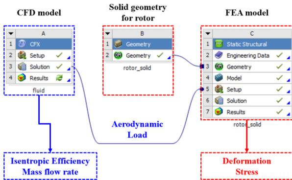
Fig. 1 Sketch for the fluid-structural interaction analysis in present study
