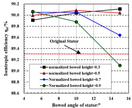
Fig. 5 Effect of bowed parameters on isentropic efficiency
