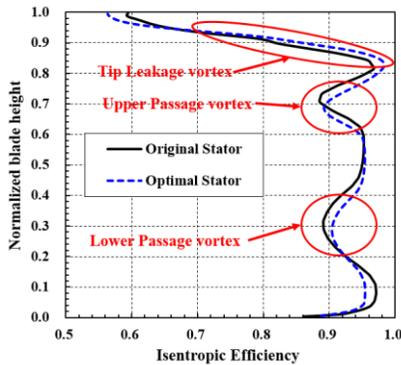
Fig. 9 Effect of bowed stator with optimal parameters on span wise distribution of efficiency
