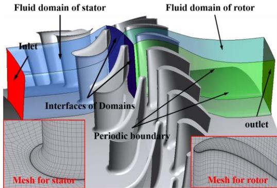
Fig. 3 CFD model of the turbine in present study
