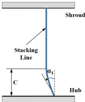
Fig. 2 Bowed parameters for stator in present study
