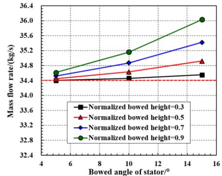
Fig. 6 Effect of bowed parameters stator on mass flow rate
