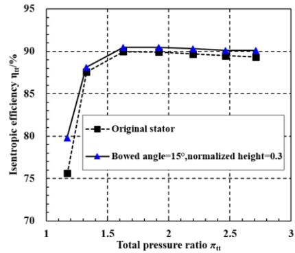
Fig. 10 Variation of  $\eta_{tt}$  with total pressure ratio
