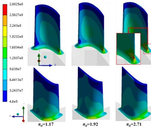
(b) Optimal bowed stator
