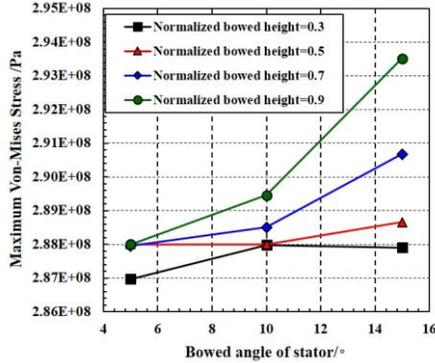
Fig. 7 Effect of bowed parameters on stress of rotor
