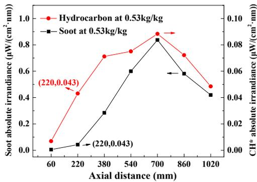
Fig 6 Axial absolute irradiances of hydrocarbon and soot at an initial PCC of 0.53kg/kg
