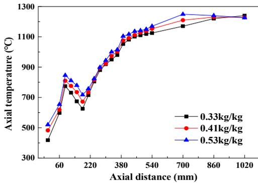
Fig 2 Axial temperatures at different initial PCCs
