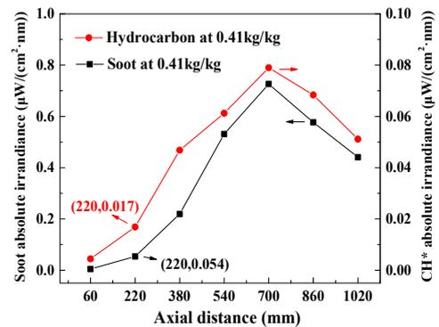
Fig 5 Axial absolute irradiances of hydrocarbon and soot at an initial PCC of 0.41kg/kg
