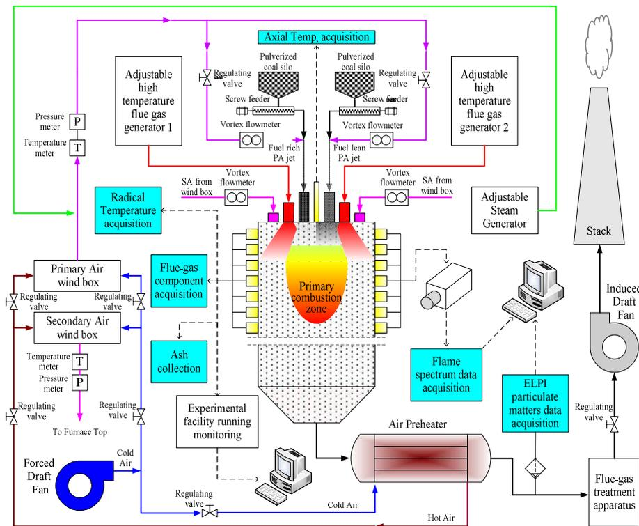
Fig 1 Schematic diagram of pilot-scale BCS system
