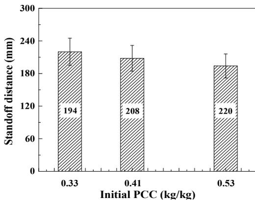
Fig 3 Standoff distances at different initial PCCs
