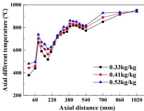
Fig 7 Axial differential temperatures at different initial PCCs
