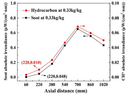
Fig 4 Axial absolute irradiances of hydrocarbon and soot at an initial PCC of 0.33kg/kg
