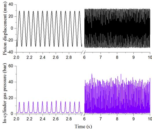
Fig 5. Experimental results of the piston displacement and in-cylinder gas pressure
