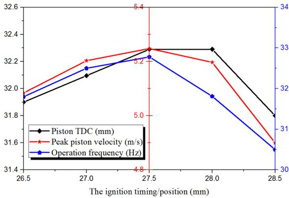
Figure 9. The piston operation parameters under various ignition timing from the experimental results
