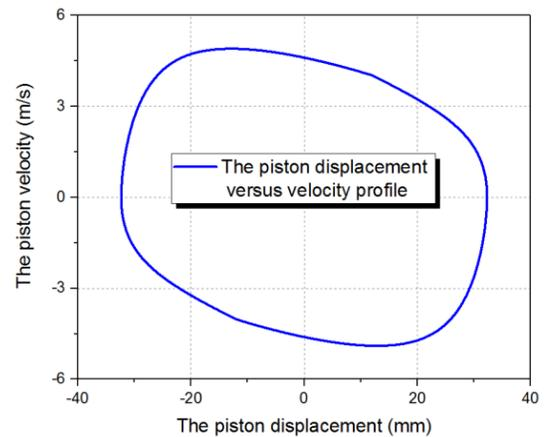
Fig 7. The processing results of the piston displacement versus velocity profile
