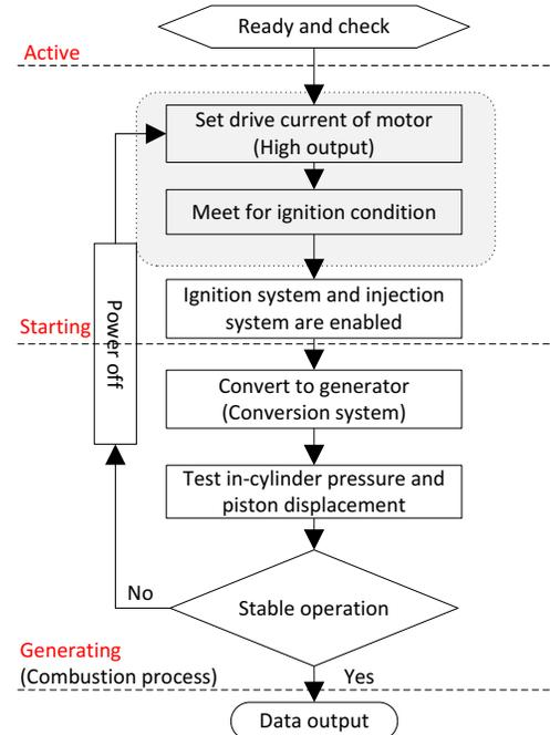
Fig 2. The FPELG operation process
