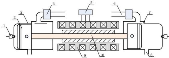
1. Spark plug 2. Piston 3. Cylinder 4. Fuel injector 5. External load 6. Air-intake tube 7. Scavenging port 8. Exhaust port 9. Stator 10. The connecting rod
