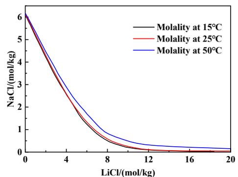
Fig 2 Solubility of the LiCl-NaCl-H<sub>2</sub>O system
