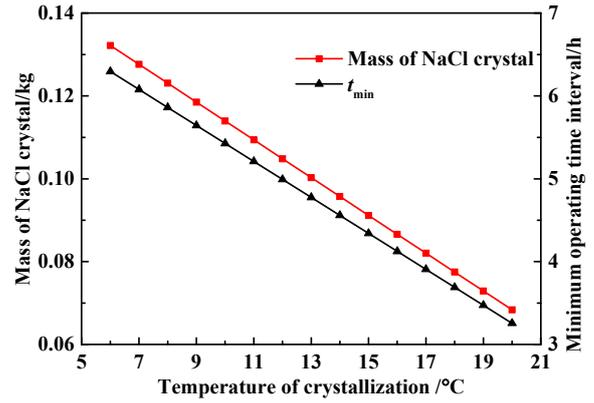
Fig 5 Effect of crystallization temperature on the NaCl separation process
