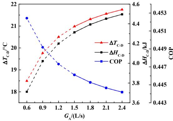
Fig 3 Effect of flow rate of solution in absorber on system performance
