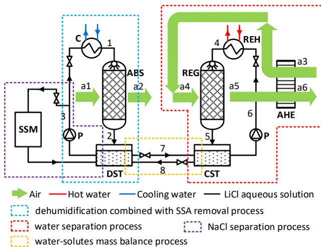
Fig 1 Flow chart of the combined liquid-desiccant dehumidification and SSA removal system driven by waste heat source
