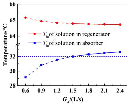
Fig 4 Effect of solution flow rate in absorber on solution temperature
