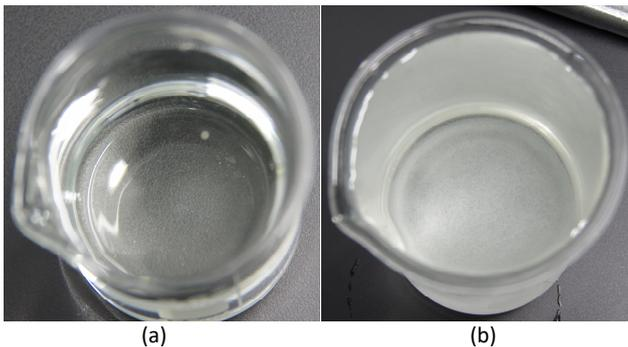
Fig 6 Change of ternary saturated solution. (a) Before cooling (b) After cooling
