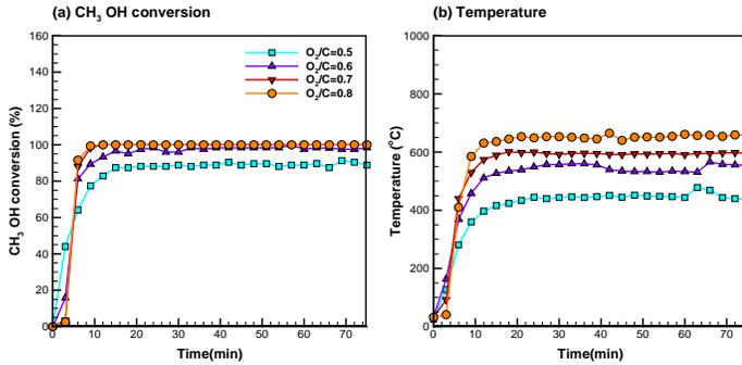
**Fig. 1.** Temporal distributions of (a) CH<sub>3</sub>OH conversion and (b) Temperature of POM at various O<sub>2</sub>/C ratios.
