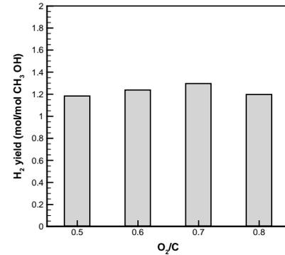
**Fig. 2.** Profiles of H<sub>2</sub> yield of POM at various O<sub>2</sub>/C ratios.
