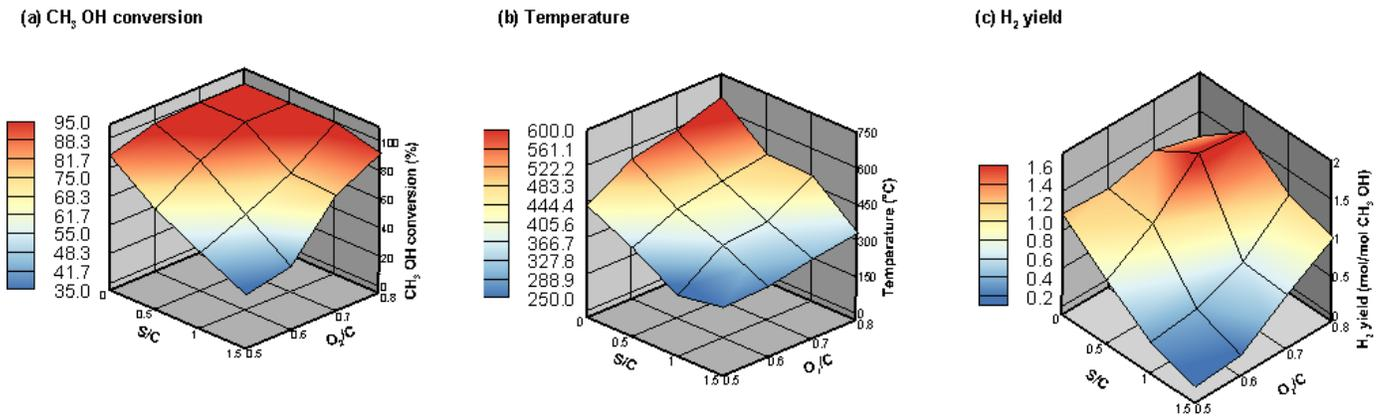
**Fig. 3.** Three dimensional profile of (a) CH<sub>3</sub>OH conversion, (b) Temperature, and (c) H<sub>2</sub> yield of ATR with various S/C ratios and O<sub>2</sub>/C ratios.
