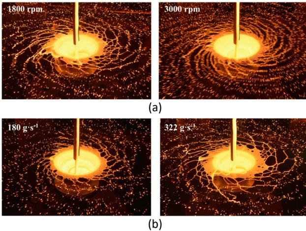
Fig 3 The structure of adopted rotary cup atomizer; (a) $Q_m=280 \text{ g}\cdot\text{s}^{-1}$ , (b) $N=1800 \text{ rpm}$ .
