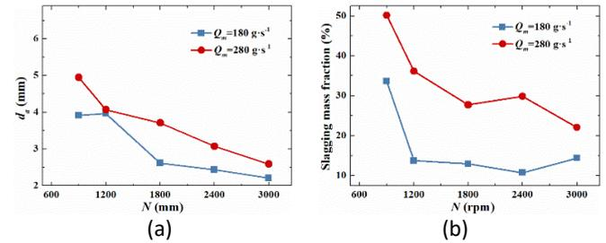
Fig 4 Effect of rotating speed on (a) average particle diameter, (b) slagging mass fraction.
