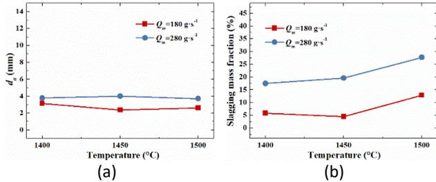
Fig 6 Effect of slag initial temperature on (a) average particle diameter, (b) slagging mass fraction.
