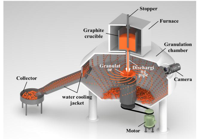
Fig 1 Schematic diagram of molten BF slag centrifugal granulation experimental system.
