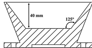
Fig 2 The structure of adopted rotary cup atomizer.
