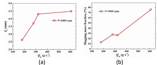
Fig 5 Effect of molten slag mass flow rate on (a) average particle diameter, (b) slagging mass fraction.
