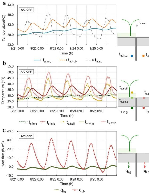
Fig. 1 Measured data of five sunny days (8/21-8/25) during the second typical period: (a) air temperatures; (b) surface temperature; (c) same for heat fluxes. (Tang and Zheng, 2019)
