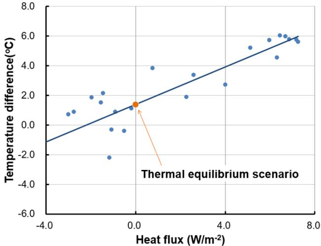
Fig. 4 Results of heat flux and indoor-outdoor air temperature difference in 24 days and the correlation between them
