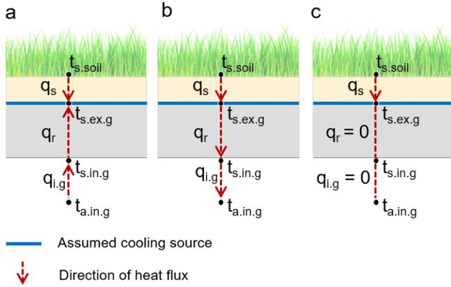
Fig. 3 Three typical heat transfer scenarios
