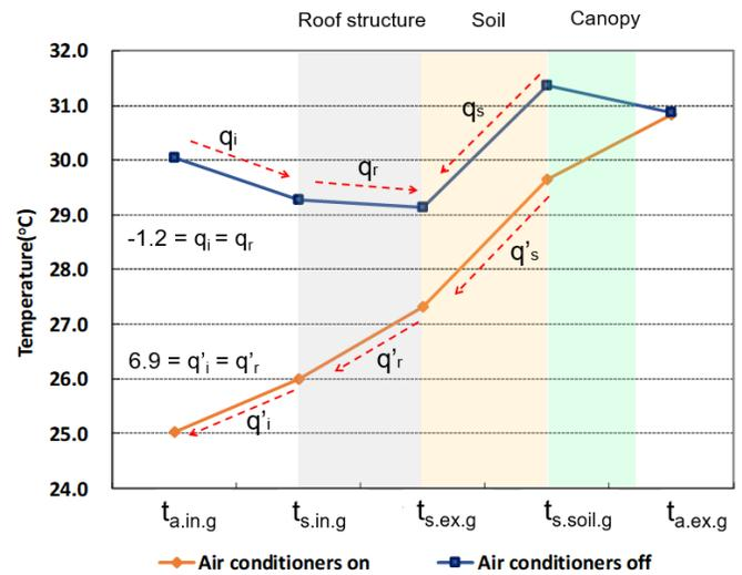
Fig. 2 Profile of average temperature of the green roof on the first typical period and the second typical period (marked as ')
