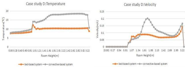
(a) Temperature comparison (b) Velocity comparison
