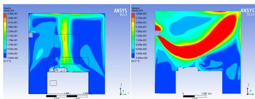
(a) Bed-based system (b) Convection-based system
