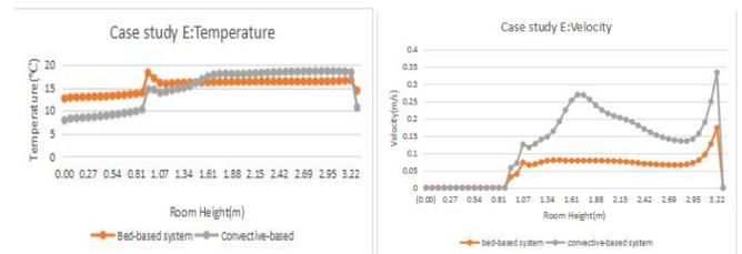
(a) Temperature comparison (b) Velocity comparison
