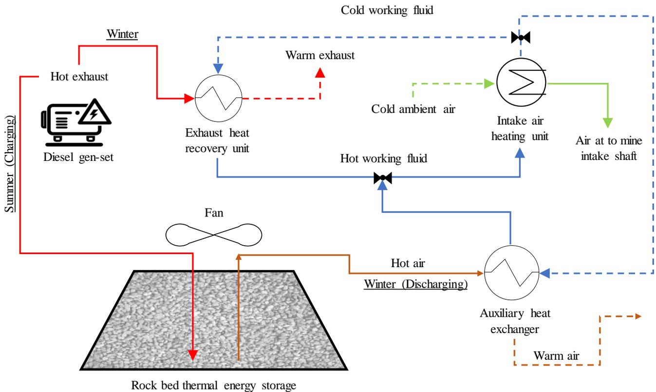
Figure 1. Schematic of the proposed system (Fluid flows have been distinguished by colors; solid and dashed lines are showing necessary heat when the energy available in the DEHR system is lower than the instant heating demand. Similarly, the DEHR system discards some of the
