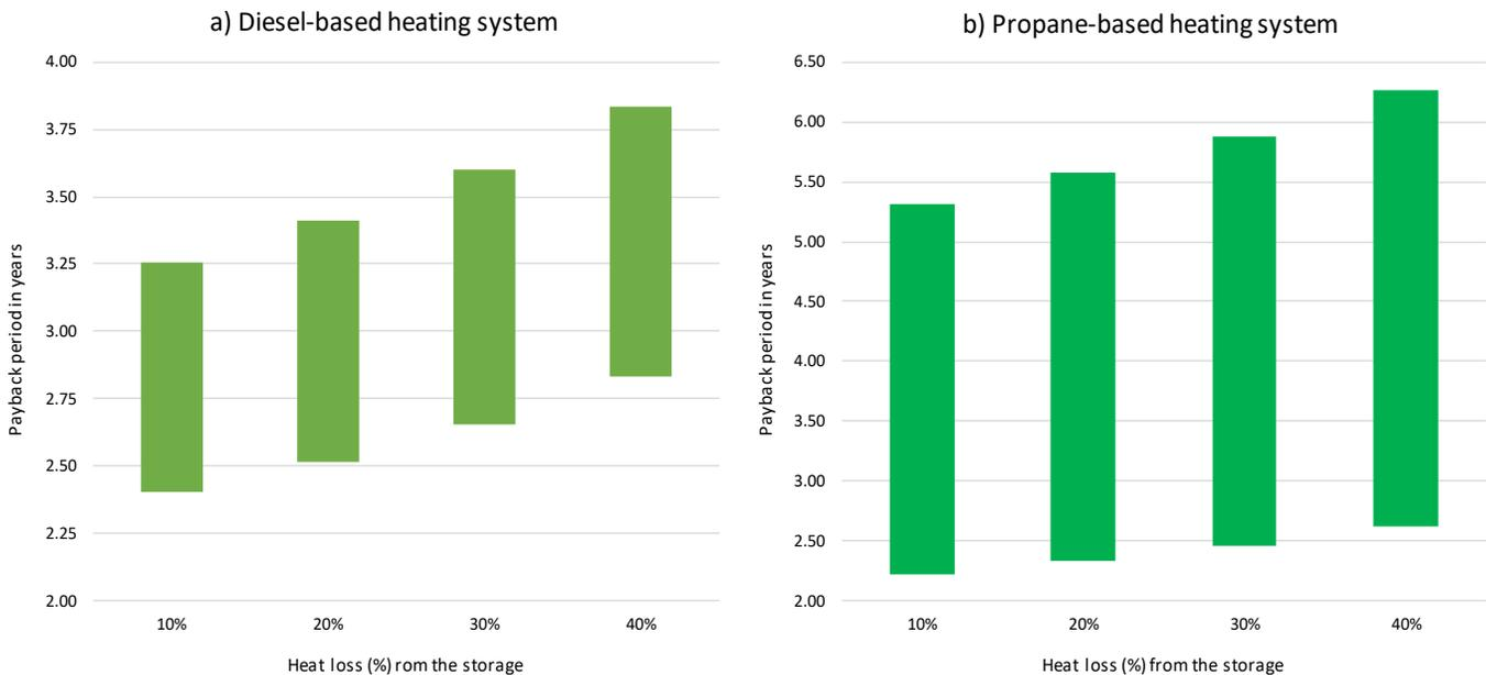
Figure 3 Range of payback periods of the DEHR-STES in a remote mine depending on the fossil fuel price
