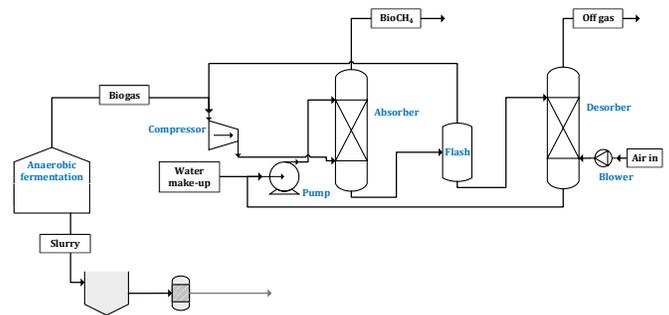
Fig 1 Process scheme of a typical HPWS
