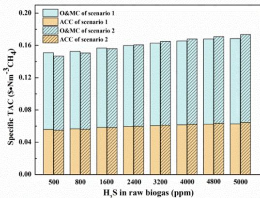
Fig 3. Specific TAC with different H<sub>2</sub>S content.
