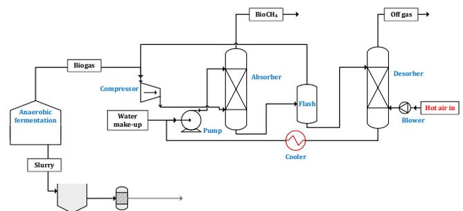
Fig 2 HPWS integrated with hot air and cooling system
