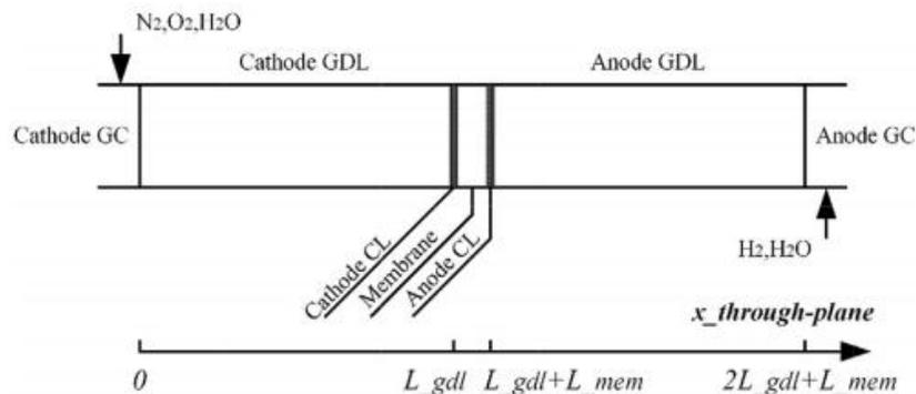
Fig 1 Schematic diagram of the one-dimensional model domains.
