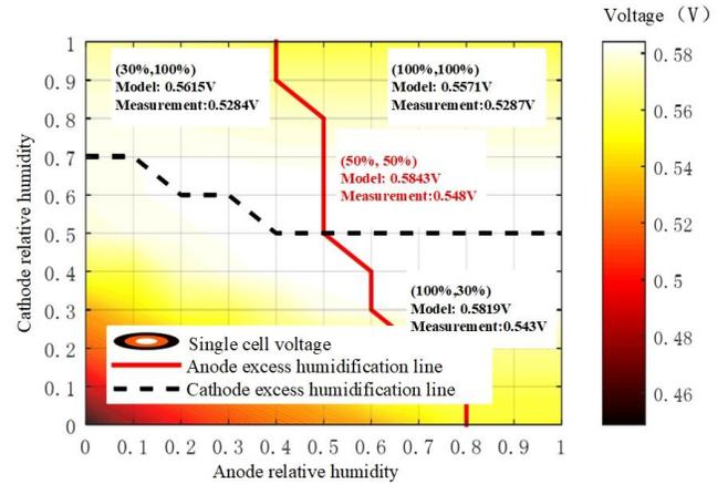
Fig 3 The single output voltage in the whole humidification plane
