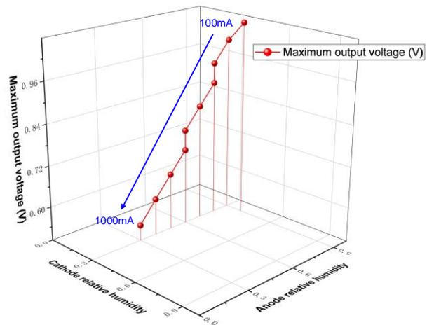
Fig 2 Maximum output voltage at different current density from 100mA/cm<sup>2</sup> to 1000mA/cm<sup>2</sup>
