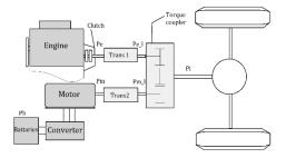
Fig. 5 Configuration of a full-size-engine parallel HEV [19]
