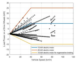
Fig. 8 Vehicle speed versus load power plane curve overlapping with load points in urban drive for 1200 kg vehicle [19]
