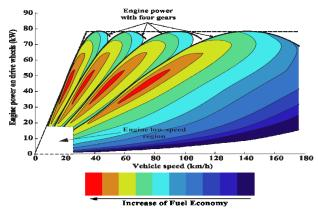
Fig. 7 Fuel consumption map for a typical 80 kW ICE in various gear ratio to the drive wheel [19]
