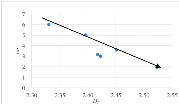
Fig. 8. The correlation between  $D_f$  and the relative permeability characteristic parameters  $n_w$
