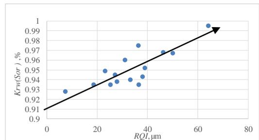
Fig. 6. The correlation between  $RQI$  and the relative permeability characteristic parameters  $K_{rw(Sor)}$
