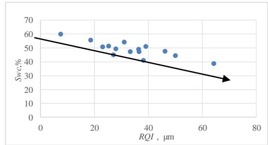
Fig. 4. The correlation between  $RQI$  and the relative permeability characteristic parameters  $S_{wc}$
