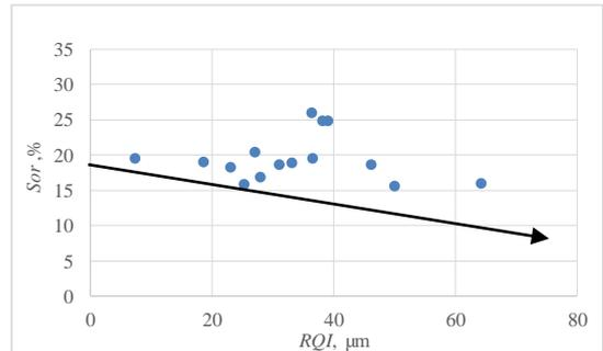
Fig. 5. The correlation between  $RQI$  and the relative permeability characteristic parameters  $S_{or}$
