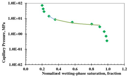
Fig. 2. The capillary pressure curve and the chosen data section
