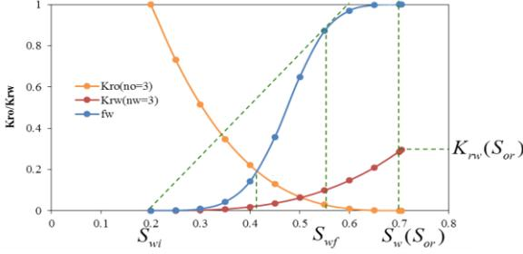
Fig. 1. The typical relative permeability curve and the corresponding characteristic parameters
