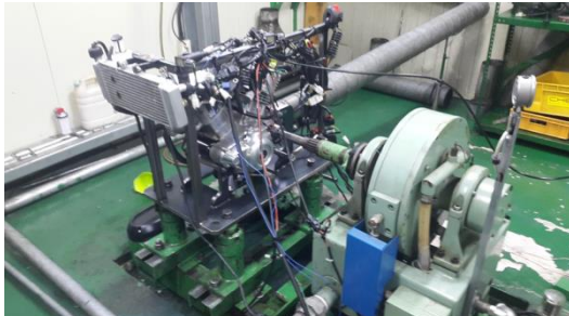
Fig 1 The the schematic of the small-SI engine testing system
