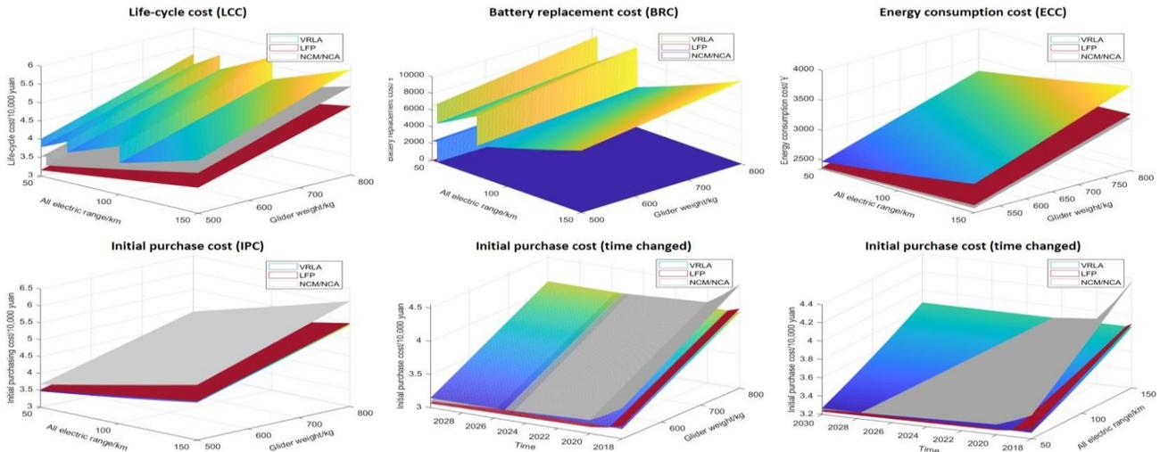
Fig 2 Life-cycle cost and different parts of it for different battery technologies, electric ranges and glider weights
