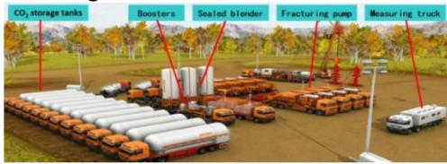
Fig.2 CO 2 waterless fracturing process
