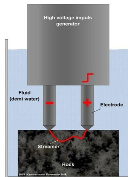
Fig. 3. Plasma-Pulse Geo-Drilling (PPGD) principle.
