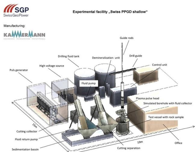
Fig. 5. Swiss PPGD experimental facility.
