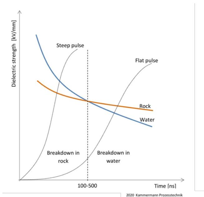
Fig. 4. Dielectric strength of water and rock versus time of pulsed voltage application [26].
