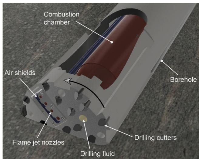
Fig. 1. The Combined Thermo-Mechanical Drilling (CTMD) technology as applied in the field (section showing inner part of drill head).
