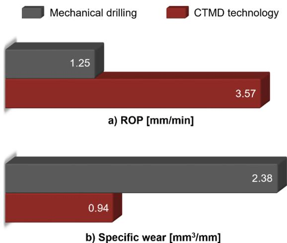
Fig. 2. Comparison of drilling performance parameters from field test: a) rate of penetration ROP; b) specific drill bit wear.
