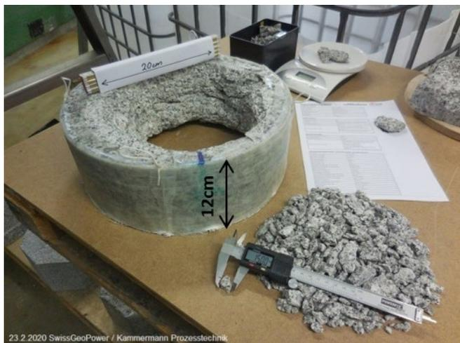
Fig. 6. Drilling results in granite using demineralized water as drilling fluid.
