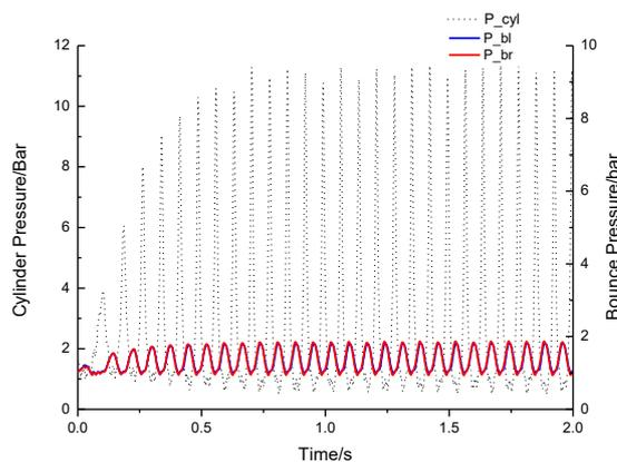
Fig.3. Pressure of combustion and bounce chamber
