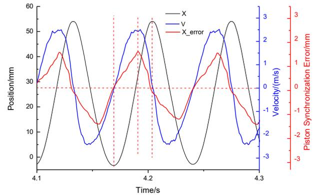
Fig.6. Piston synchronization error along with position and velocity
