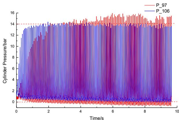
Fig.7 Cylinder pressure of various control method
