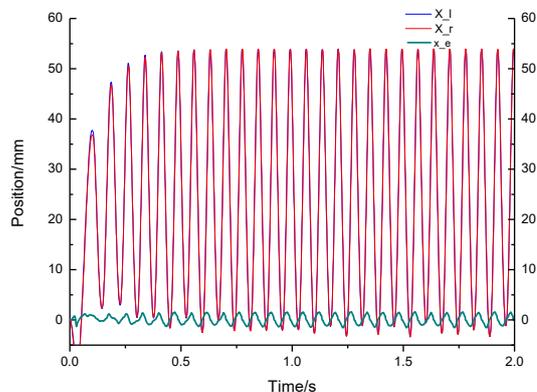
Fig.2. Positon and synchronization error of the opposed piston
