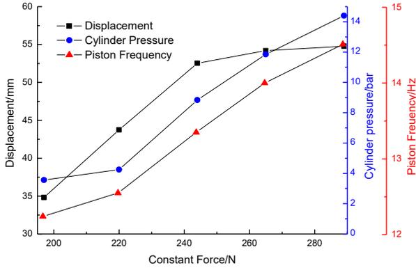
Fig.4. Piston displacement and frequency, cylinder pressure for various constant force
