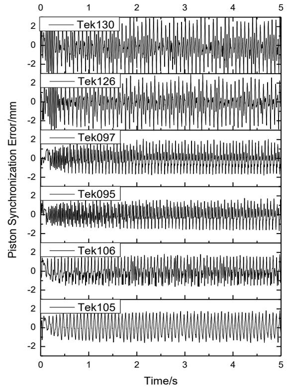
Fig.5. Piston synchronization error under difference control strategies
