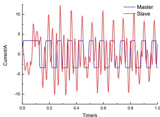
Fig.8 Target current of the mater and slave motor
