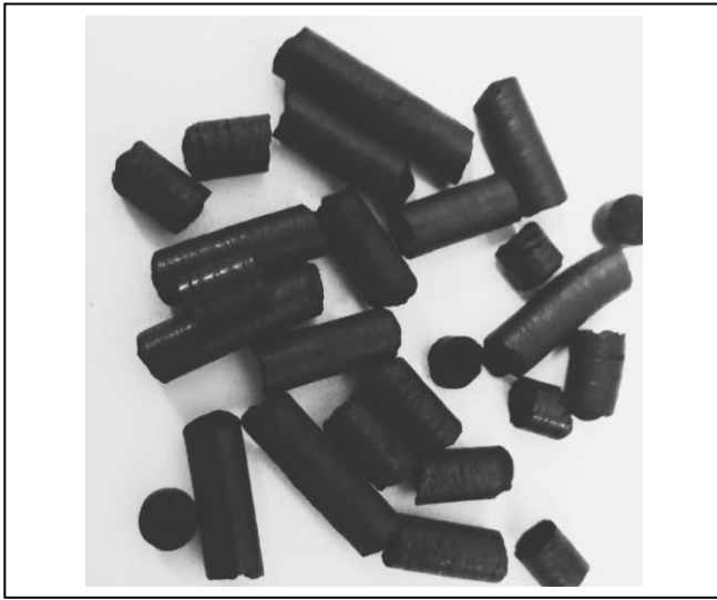
Fig. 2. Biocarbon pellet produced at the University of Perugia
