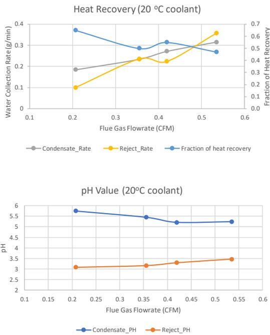
Fig. 5 Impacts of flue gas flow rate (at 148 °C membrane HX inlet temperature, 20 °C coolant).
