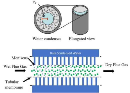
Fig. 1 Capillary condensation principle: (a) concave meniscus; (b) condensation through membrane.
