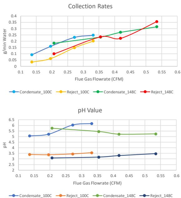
Fig. 6 Impacts of membrane HX inlet temperature (at 20 °C coolant).
