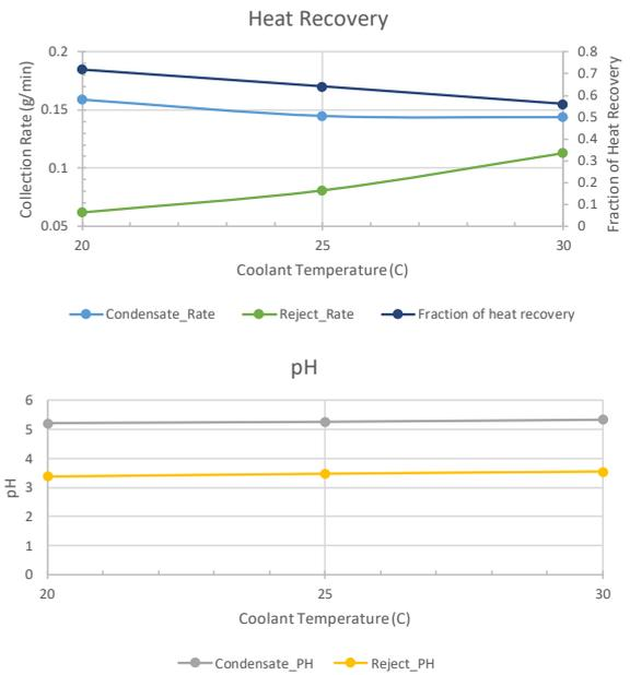
Fig. 7 Impacts of coolant temperature (at 100 °C membrane HX inlet temperature, 0.2 cfm flue gas flow rate).
