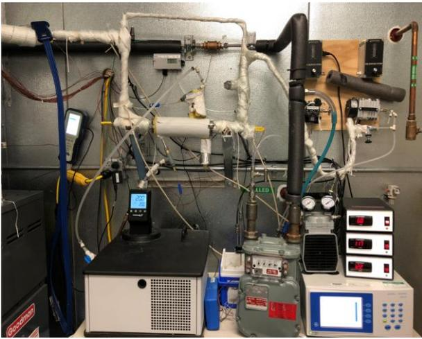
Fig. 3 Testing system for the membrane heat exchanger.
