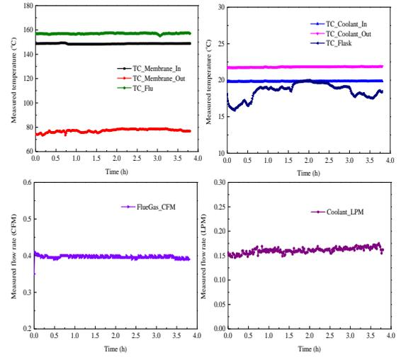
Fig. 4 Measured data during a typical test on the membrane heat exchanger.
