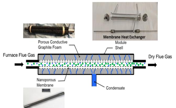
Fig. 2 Membrane-based condensing heat exchanger developed in this study.
