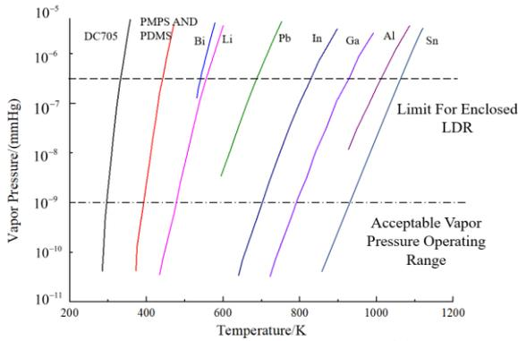
Fig.2 Candidate working mediums for LDR system
