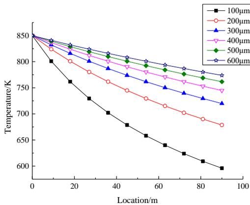
Fig.3 Droplet temperature over movement distance at different droplet radii
