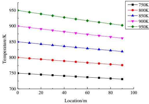
Fig.7 Droplet temperature at different initial temperature
