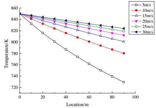
Fig.5 Droplet temperature over movement distance at different velocities
