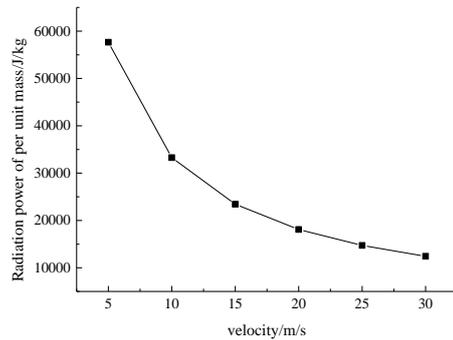
Fig.6 Variation of unit mass radiation with different velocity
