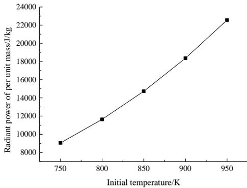
Fig.8 Radiation power per unit mass over the droplet initial temperature
