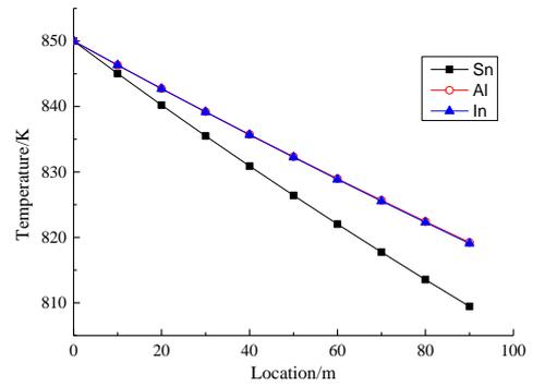
Fig.9 Temperature changes of droplets with different mediums
