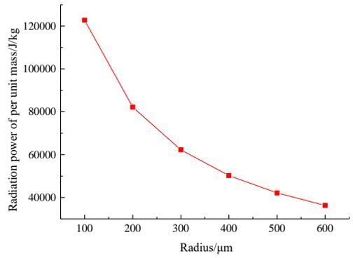
Fig.4 Radiation power per unit mass over droplet radii
