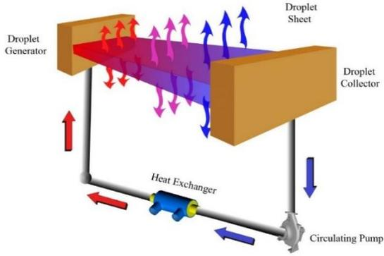
Fig.1 Schematic of the droplet radiation radiator
