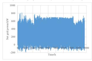
Fig. 4(b) Net grid power of the system without battery storage
