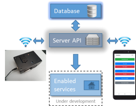
Figure 3 Comfort Platform: basic communication layout
