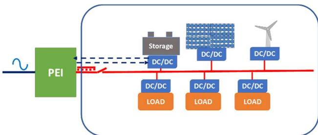
Fig 6 PEI-Storage virtual inertia service to AC frequency regulation
