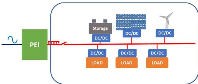
Fig 3 PEI-MG schematic representation
