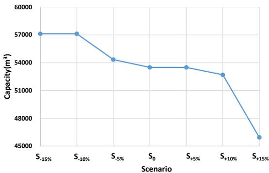
Fig 3 Pipeline capacity for transporting biofuel under different scenarios.
