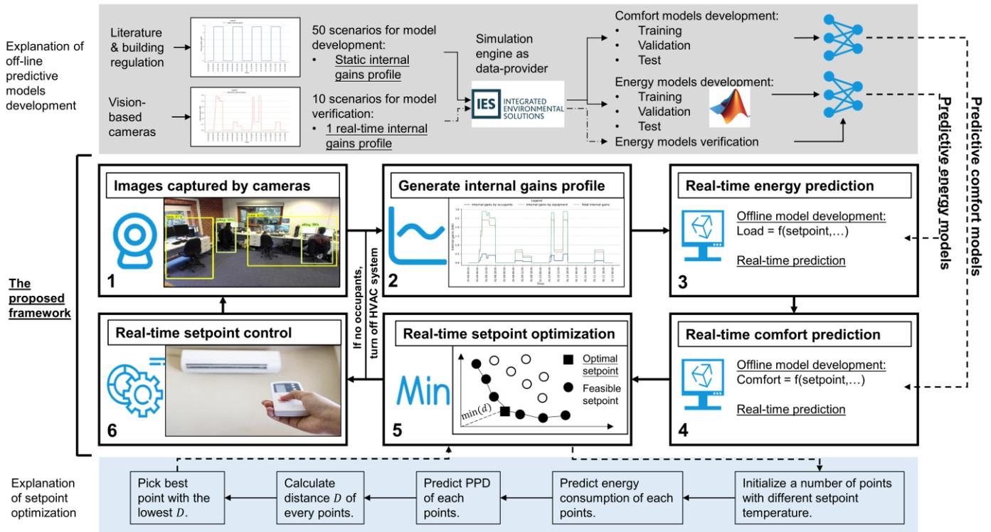
Fig 3 The integrated framework: real-time internal gains identification and HVAC setpoint optimization
