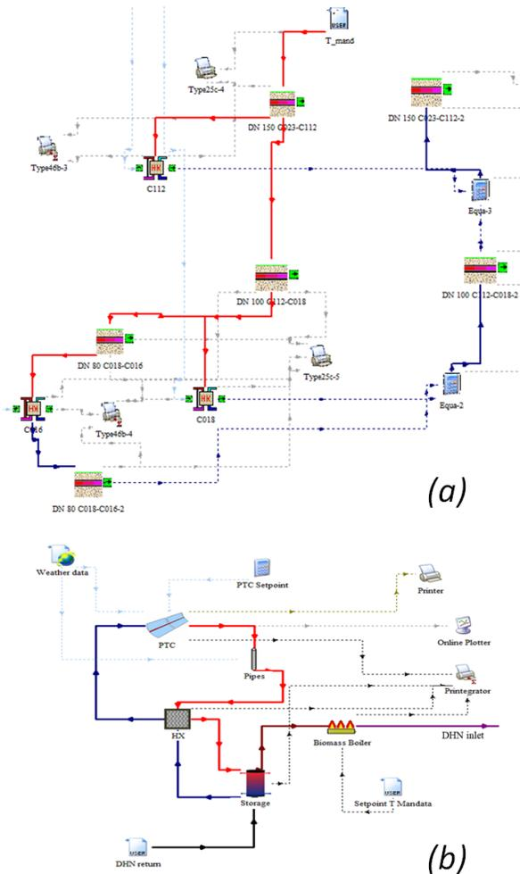
Fig 2 (a) model of the DH. (b) model of the heating plant
