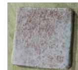
Fig.7. Copper foam /paraffin composite phase change material with a porosity of 85% and a pore density of 50 ppi was prepared.
