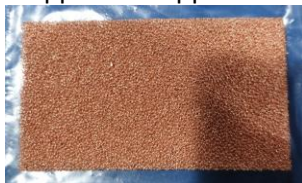
Fig. 4. Copper foam with a porosity of 85% and a pore density of 50 ppi.
