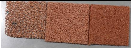
Fig. 3. Copper foam with a porosity of 95% and a pore density of 15 ppi, 30 ppi and 50 ppi.
