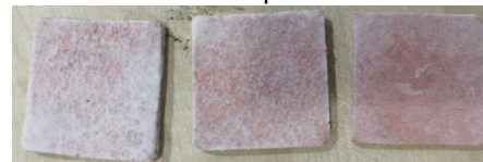
Fig. 6. Three copper foam /paraffin composite phase change materials with a porosity of 95% and a pore density of 15 ppi, 30 ppi and 50 ppi from left to right were prepared.
