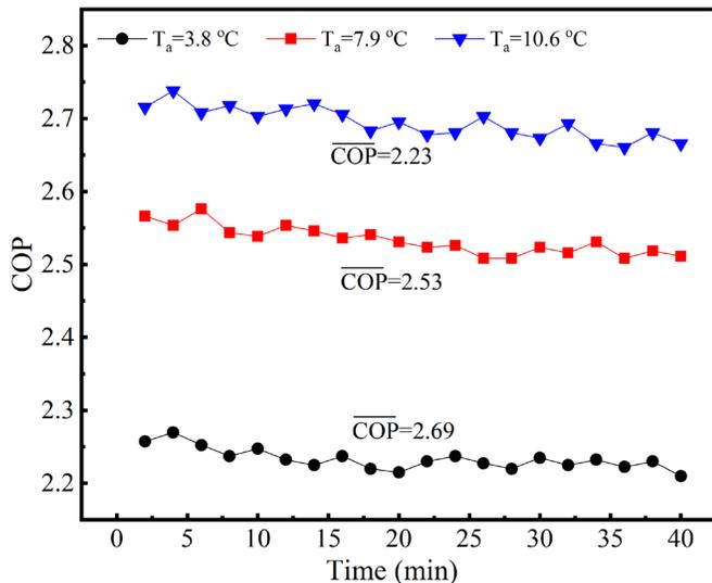
Fig 7 The variation of COP at different ambient air temperature.
