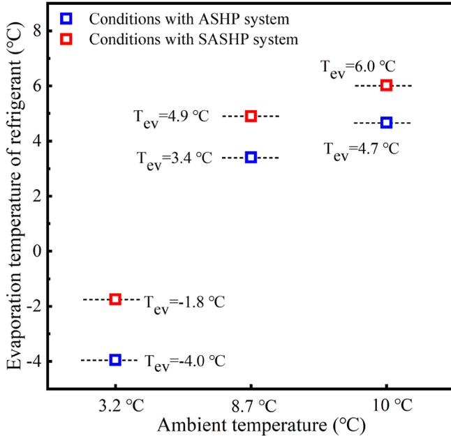
Fig 4 The evaporation temperature of different conditions.
