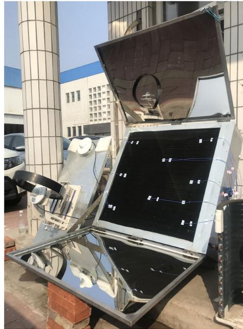
Fig 1 Structure of the collector-evaporator.
