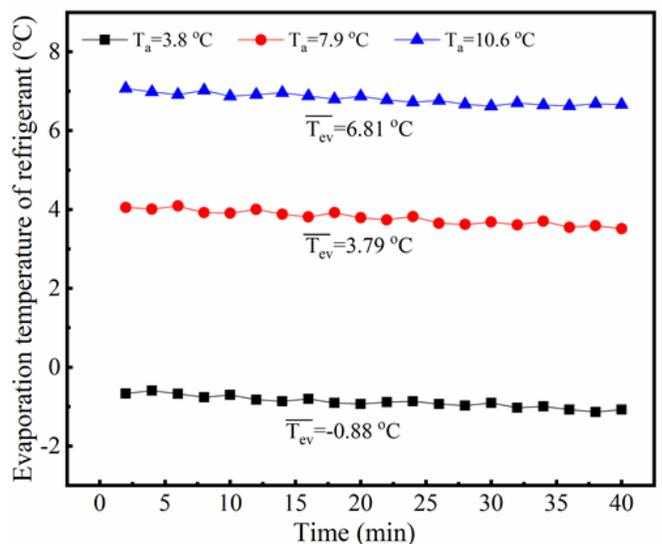
Fig 6 The variation of the evaporation temperature of refrigerant at different ambient air temperature.
