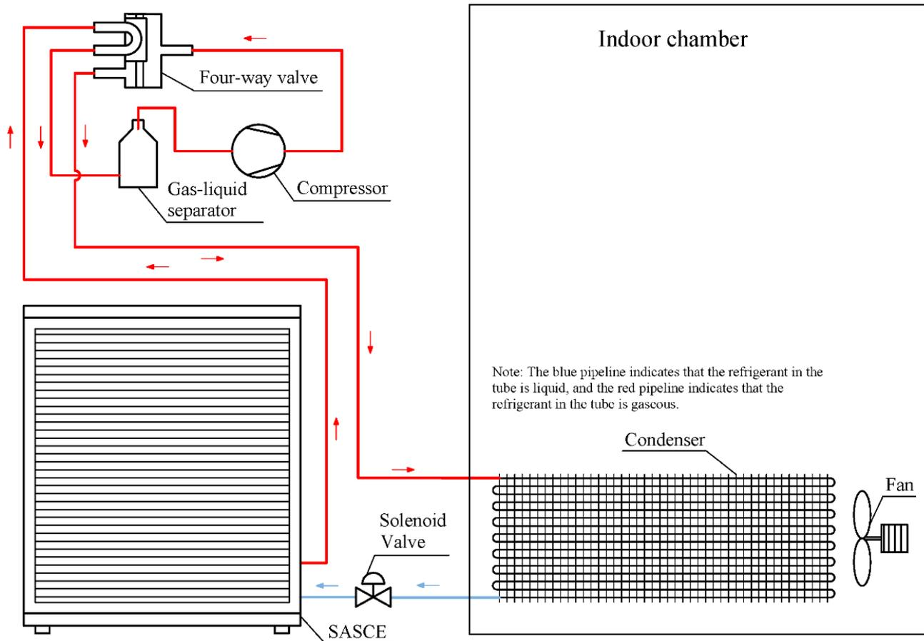
Fig 3 Schematic diagram of the SASHP system.
