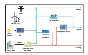
Fig 1 Schematic representation of a renewable multi-energy system.
