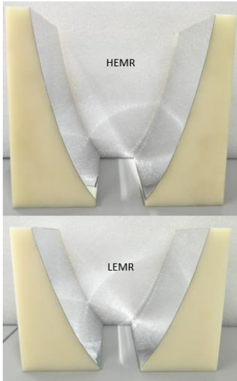
Fig. 3 Pictures of 3-D printed HEMR (up) and LEMR (down)
