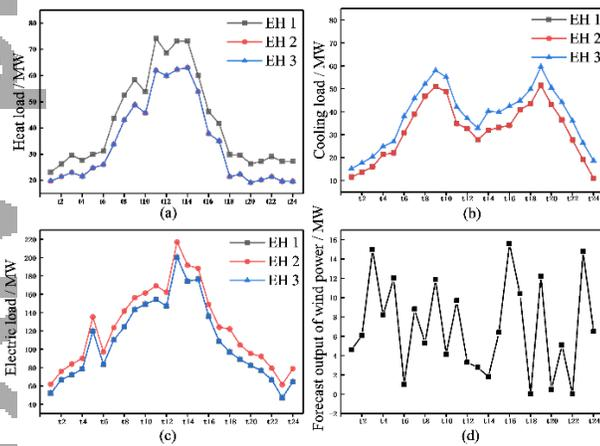
Fig3 variation curve of load and wind power: (a) heat load; (b) cooling load; (c) Electric load; (d) Forecast output of wind power
