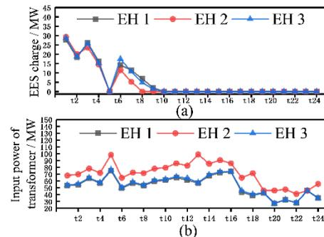
Fig 5 The distribution of Input electricity: (a) EES equipment inputs electricity every hour; (b) Power input of transformer per hour
