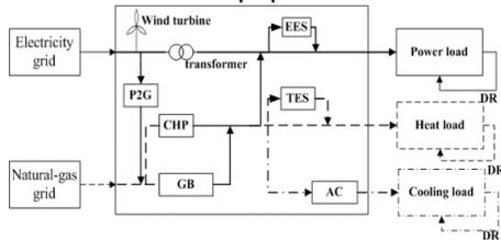
Fig 1 the energy hub in the multi-energy hub system
