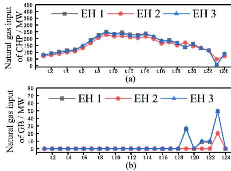
Fig 7 the distribution of natural gas; (a) CHP unit inputs natural gas per hour; (b) Natural gas input of GB
