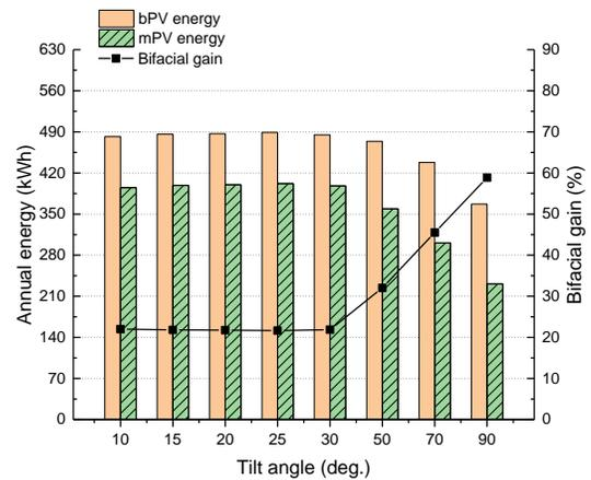
Fig. 10 The effect of tilt angle on bPV and mPV performance.
