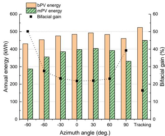
Fig. 9 The effect of orientation on the PV performance.
