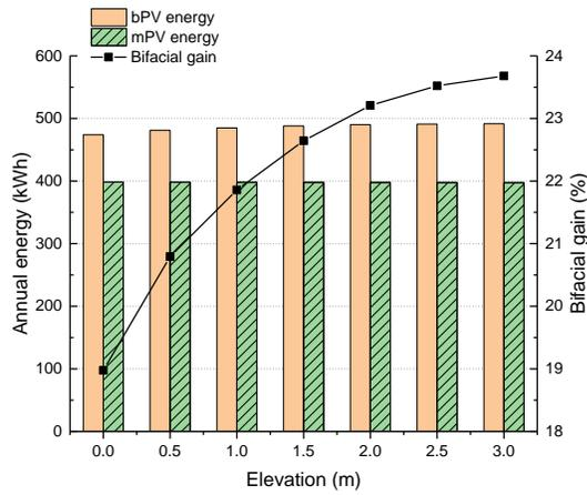
Fig. 11 The effect of elevation on bPV and mPV performance.
