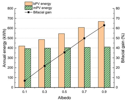
Fig. 8 The effect of ground albedo on the PV performance.
