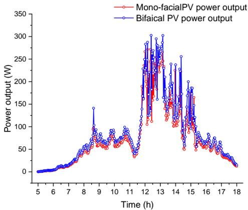
Fig. 4 Power output of mPV and bPV modules on the day. For better characterization, bifacial gain versus time is presented in Fig. 5 to show the advantage of bPV technology. The bifacial gain is fluctuated and ranged from 0-40% on the day. The average bifacial gain is up to 17.33%.
