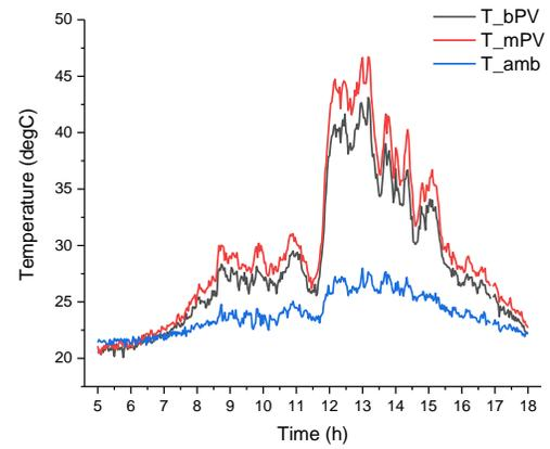
Fig. 6 Ambient temperature and PV cell temperature.
