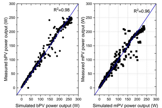
Fig. 3 Validation of bPV and mPV performance.
