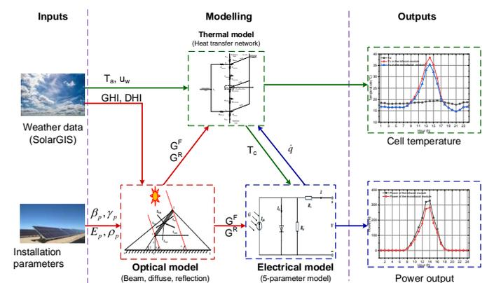
Fig. 1 A framework for simulating the bPV performance [12].
