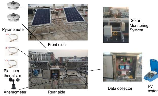
Fig. 2 Configuration of the bPV experimental system.
