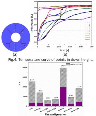
Fig.5. Total melting time and bottom melting time.
