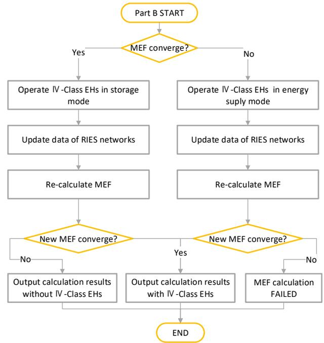
Fig 5 Algorithm part B flow chart
