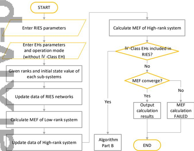
Fig 4 MEF calculation algorithm flow chart
