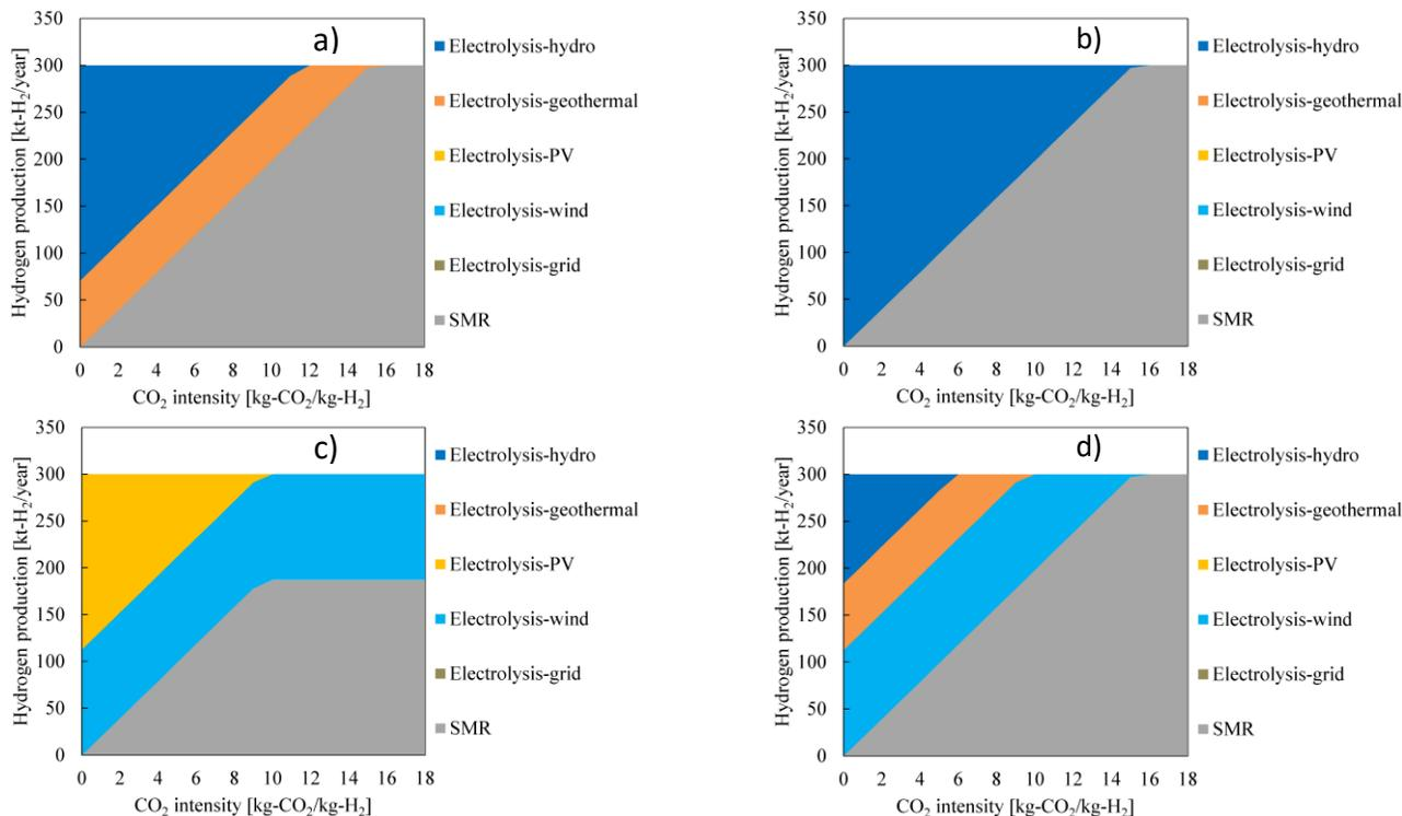
Fig 1 Hydrogen production system configuration. a) LC scenario; b) LEU scenario; c) WEC scenario; d) WECC scenario.
