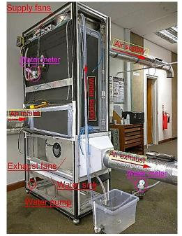
Fig. 1 Experimental rig for dew point evaporative cooler
