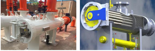
Fig 1 Physical appearance and internal structure of horizontal gas filter
