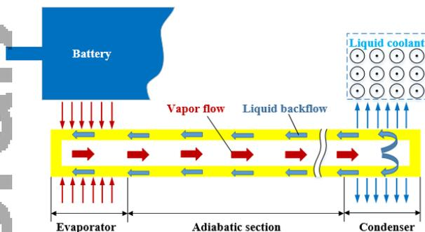
Fig 2 Heat transfer process of the BTMS
