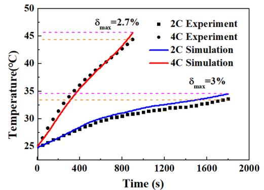
Fig 4 Model validation for the proposed BTMS
