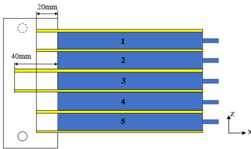
Fig 6 Variable heat pipe length optimization scheme
