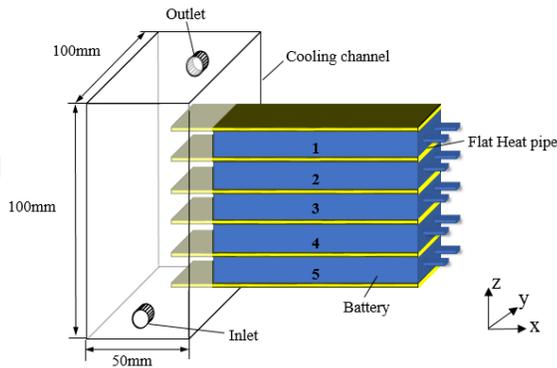
Fig 1 Schematic illustrations of the BTMS
