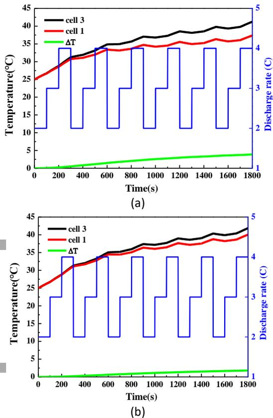
Fig 8 Temperature trend comparison during the current changing discharge process: (a) original; (b) optimized
