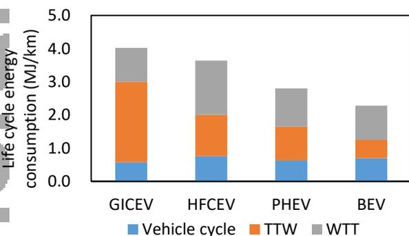
Fig 2 Life cycle energy consumption of vehicles
