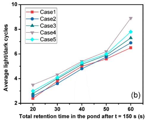
Fig 10 (a) Average retention time in the light zone, and (b) Average light/dark cycles at cases with different dam lengths
