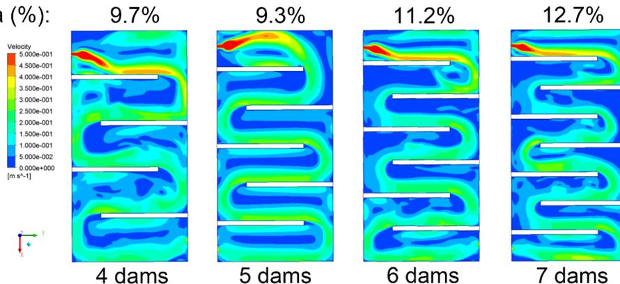
Fig 6 Velocity contour and dead zone area in the plane of  $z = 18$  mm
