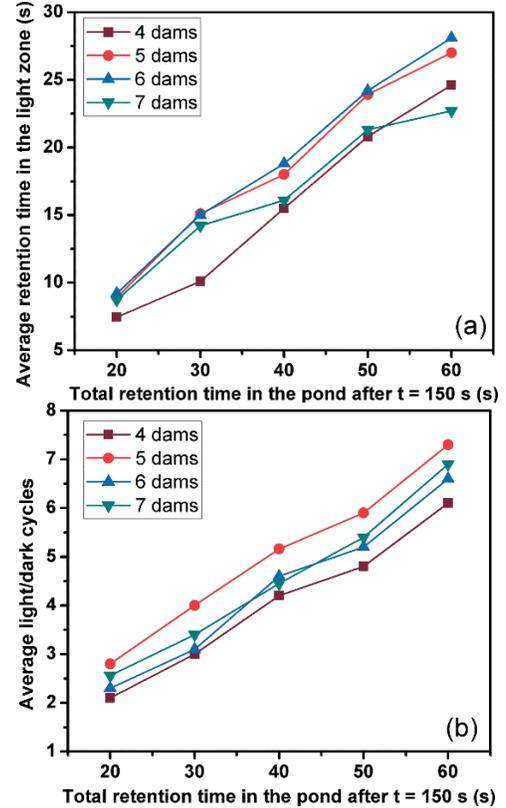
Fig 7 (a) Average retention time in the light zone, and (b) Average light/dark cycles at cases with different dam numbers
