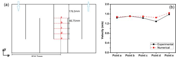
Fig 5 (a) Locations of the experimentally measured points, and (b) Numerical validation
