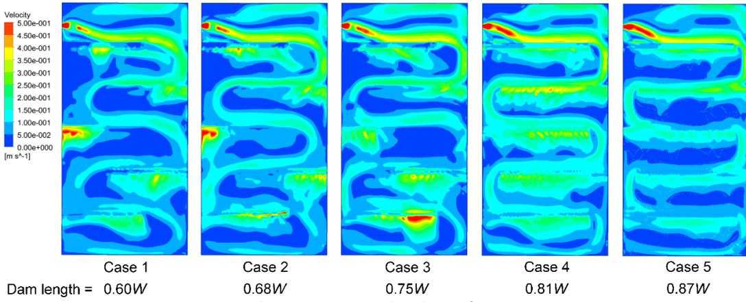
Fig 8 Velocity contour in the plane of  $z = 38$  mm
