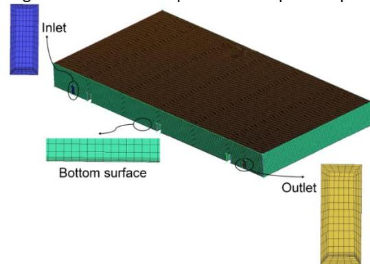
Fig 2 Grid meshing of the pond model
