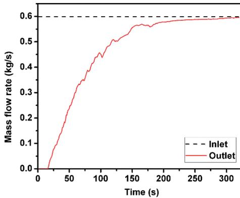
Fig 3 Variation of the mass flow rate in the outlet
