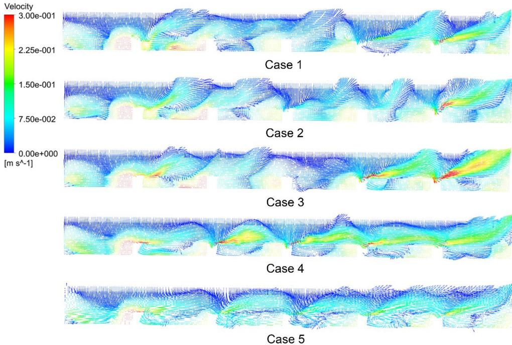
Fig 9 Velocity vector in the plane of  $y = 350$  mm
