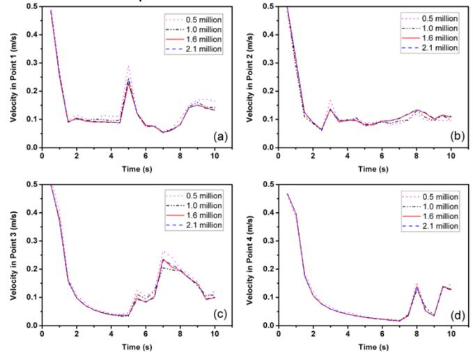
Fig 4 Grid sensitivity study for points 1 to 4 in the pond
