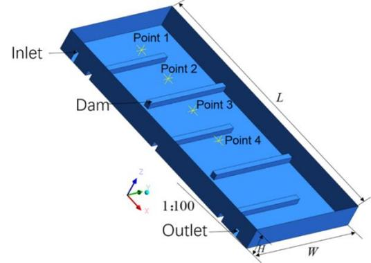
Fig 1 Schematic of the pond with serpentine path
