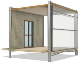
Fig 2 Design concept of the double-glazed external facade
