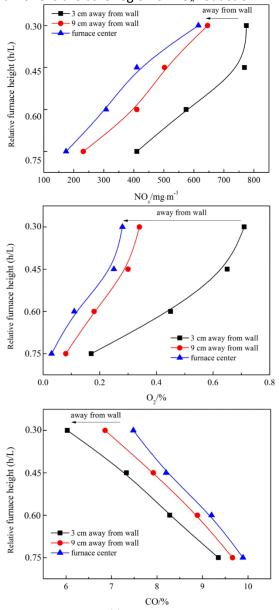
Fig 4 The distribution of flue gas components in the radial direction of the cyclone barrel.
