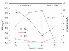
Fig 3. The distribution of flue gas components along the direction of flue gas flow
