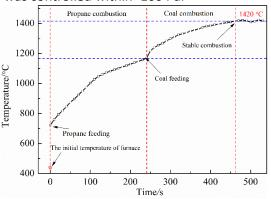
Fig 2 Temperature changes of flue gas in cyclone barrel
