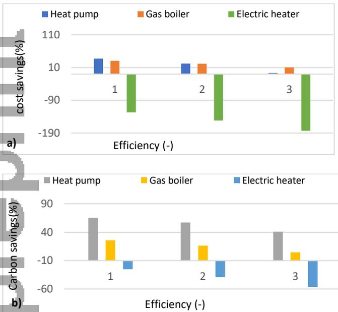
**Fig. 4.** Savings (%) considering oil boiler at 80% efficiency as a base case, a) cost, b) carbon emission.
