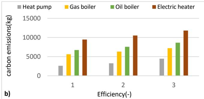
**Fig. 3.** a) Seasonal cost and b) Carbon emission against the efficiency for the HP, oil gas boiler technology for the three cases with efficiency of 90, 80 and 70%.
