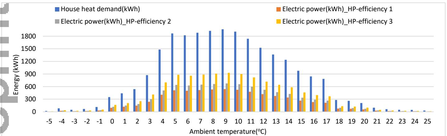
**Fig. 2.** The heat demand (space heating and DHW) with electric power consumption in each bin.
