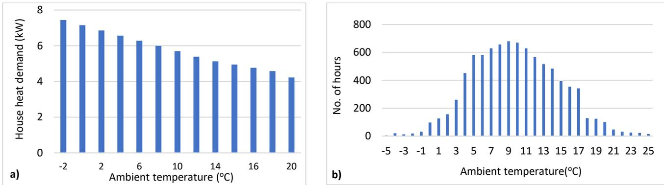
**Fig.1.** Case study under consideration, a) House heat load demand, b) Experienced number of hours at different ambient temperature conditions for Belfast, UK.
